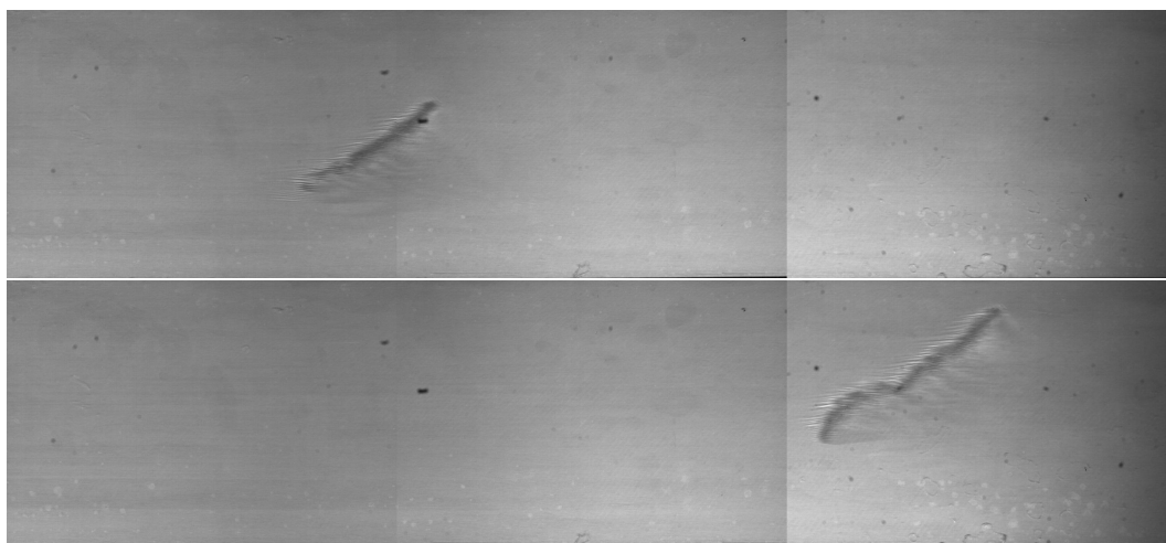
Figure 1. Experimental realisation of growing turbulent stripes at Re=750 based on the centreline velocity, as time goes by (flow from left to right).
